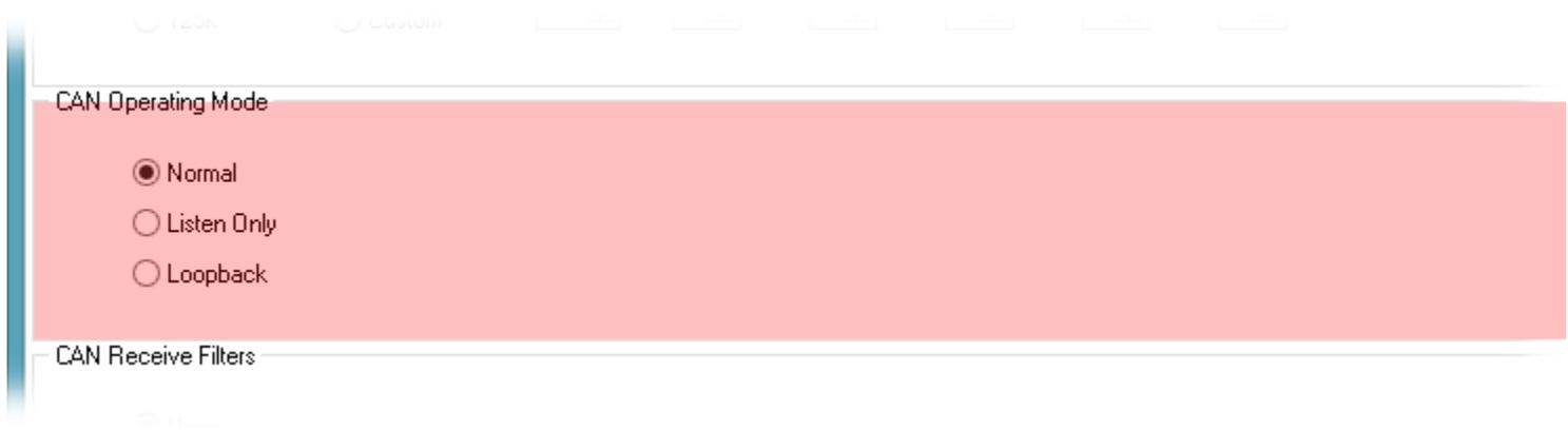
'Normal' mode, allows full transmission & reception of CAN messages & is the normal mode of operation. In this mode, the CANdo device operates as an active CAN node on the CAN bus, meaning that it responds to valid messages with an acknowledgment, as per the CAN bus standard.
